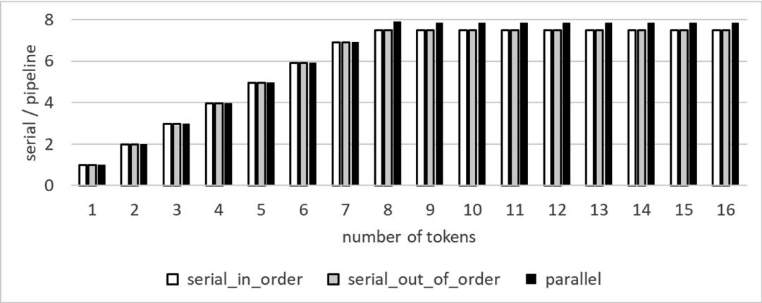
Figure 11-46. The speedup achieved by the different filter execution modes when executing a balanced pipeline with eight filters, 8,000 items, and an increasing number of tokens. The filters spin for 100 microseconds. Collected on our Linux Server System. Sample code performance_tuning/parallel_pipeline_timed.cpp
