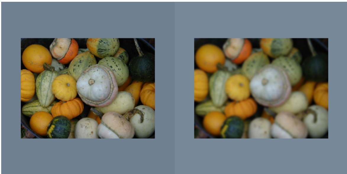
Original image (left). Convolution (right): f \star k(x, y) = \sum_{i,j} f(i, j)k((x - i), (y - j)) (GaussianSmooth.cxx or GaussianSmooth.py)
