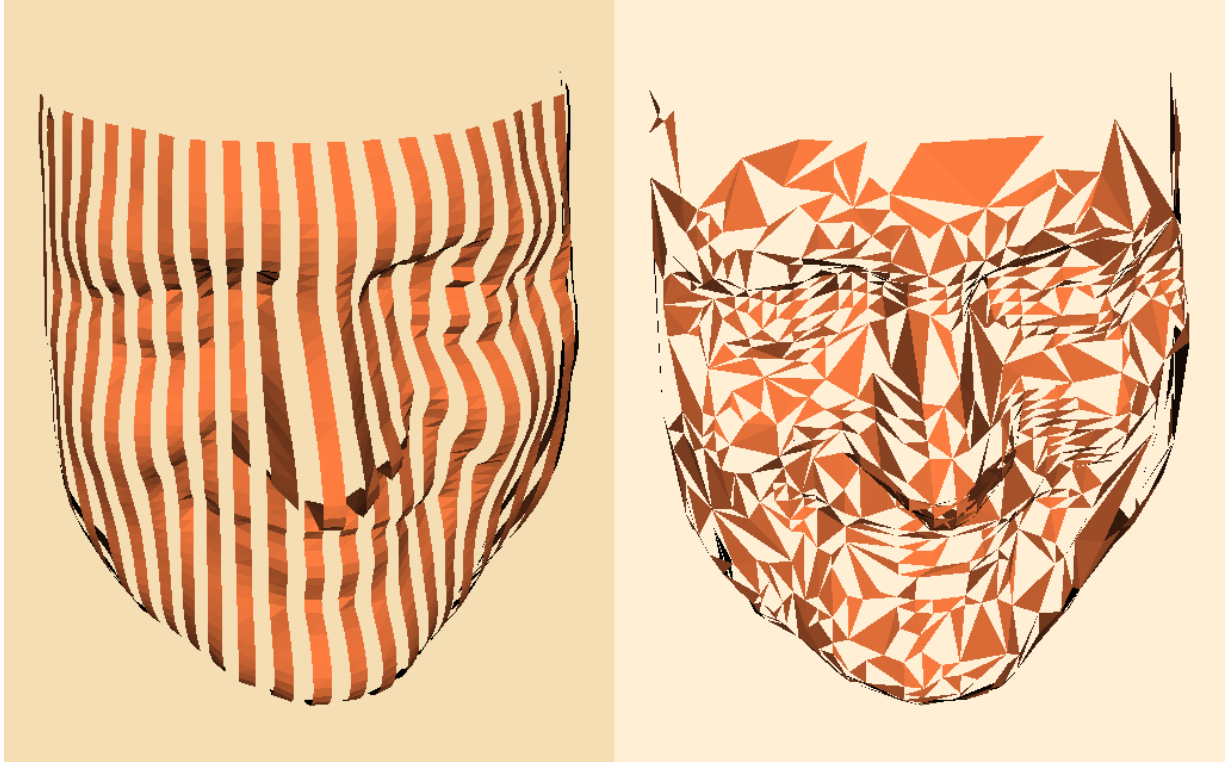
Figure 9.21: Triangle strip examples. Left, structured triangle mesh consisting of 134 strips each of 390 triangles. Right, Unstructured triangle mesh consisting of 2227 strips of average length 3.94, longest strip 101 triangles. Images are generated by displaying every other triangle strip. ( StripFran.cxx or StripFran.py )
