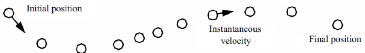
Figure 6.16: Time animation of a point C . Although the spacing between points varies, the time increment between each point is constant.
