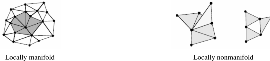
Figure 8.27: Manifold and nonmanifold surface topology. If the local neighborhood around a vertex is topologically a 2D disk (i.e., a small disk can be placed on the surface without tearing or overlapping), then the surface is manifold at that vertex.
